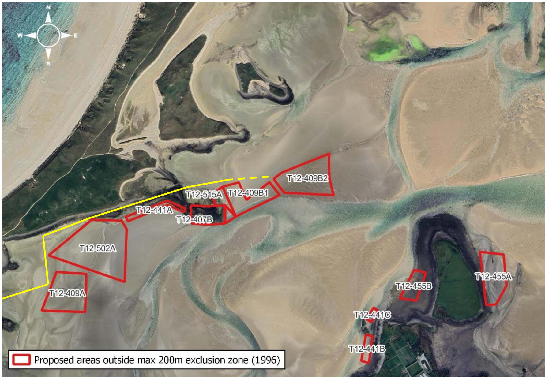
Revised Seal Haul Out 200m buffers based on georeferenced satellite imagery (1996) Route as per licence application (yellow) Estimated additional route (yellow dash)
